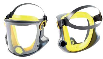
The newly developed Multimask Pro has a redesigned face seal made of silicone which ensures greater comfort for the wearer, quicker cleaning and a higher protection class. Thanks to the special mask frame the user has the possibility to control the airflow in the headpiece. The headpiece is fitted with a removable cellulose acetate visor treated with a durable anti-fog varnish to ensure a permanent free vision.
